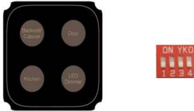
Figure 2 The right dip switch setting of WMSP4
